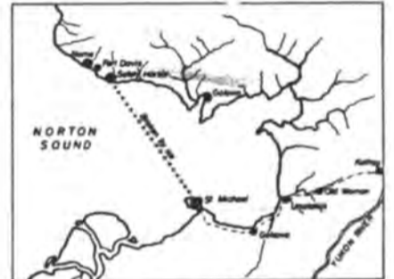
Map showing the wireless circuit between Nome and Fort St. Michael, Alaska, a distance of 100 miles. This circuit was put into operation by the U.S. Signal Corps in 1903 to replace the cable which was washed out by ice every year.
